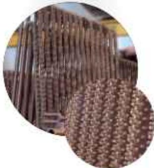
Studded in-bed evaporator tubes are immersed in-bed to extract heat
